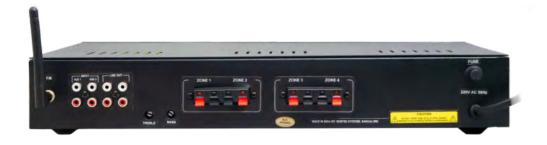
2 Zones x 50 watts @ 8 Ohms Class D High performance Amplifier with independent volume control for 2 zones | Connect upto 4 speakers (8 Ohms) without LMT | Built in USB & SD Card reader- MP3/WAV, Bluetooth, FM Tuner Dimension: 17 inch x 8 inch x 2.5 inch
